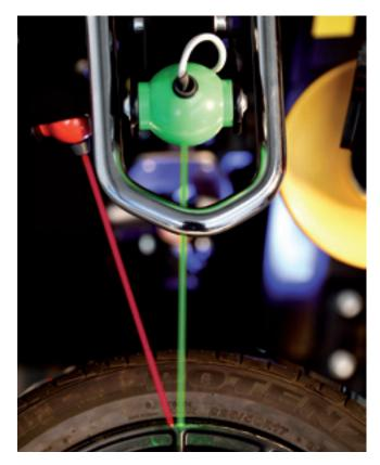
Two laser pointers determine the wheel size
