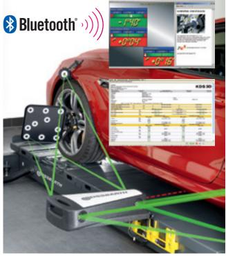
3D sensor heads and measurement boards in action
