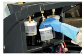
Hermetically closed oil and UV-dye bottles ensure moisture free and clean storage
