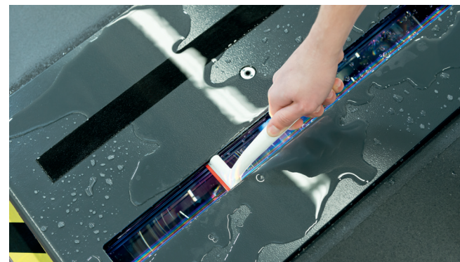
The measuring strip can be cleaned from the outside without opening mechanical components
